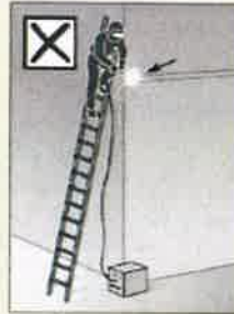
(a) Performing hot work from ladder
