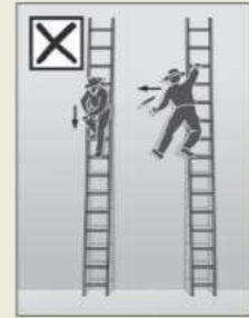
(d) Facing away from the ladder to descend; over-reaching
